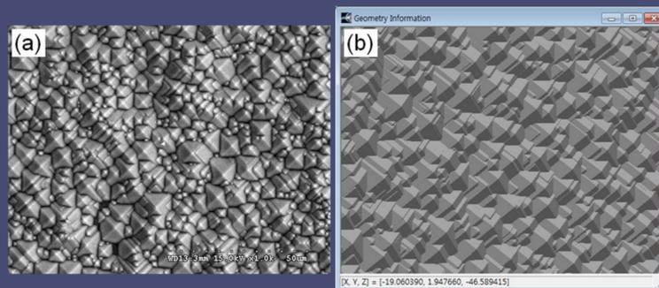
Fig. 4. (a) Surface morphology of textured Si sample. (b) 3-D rendering image of the geometric information for simulation.
