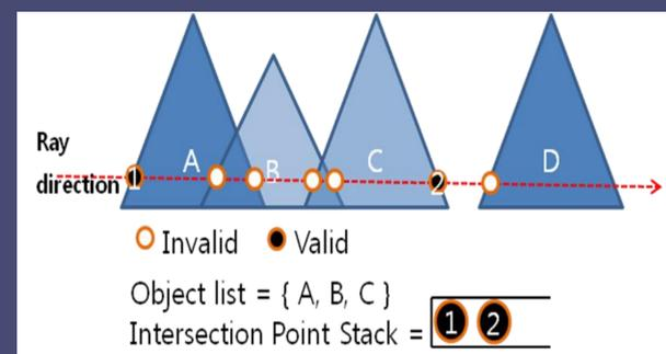
Fig. 2. Schematics of logic for finding intersection points between objects and ray.
