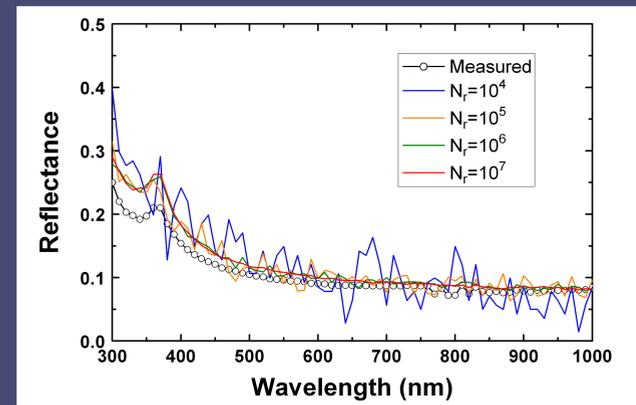
Fig. 5. Comparison of measured and simulated reflectance spectra.
